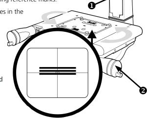
Securing the stage (150mm x 100mm & 200mm x 100mm)
