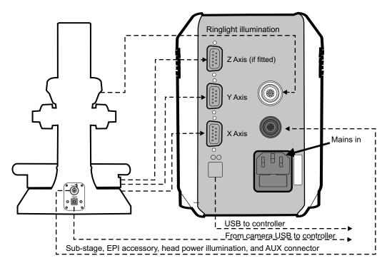
All connectors must be engaged fully and secured.
